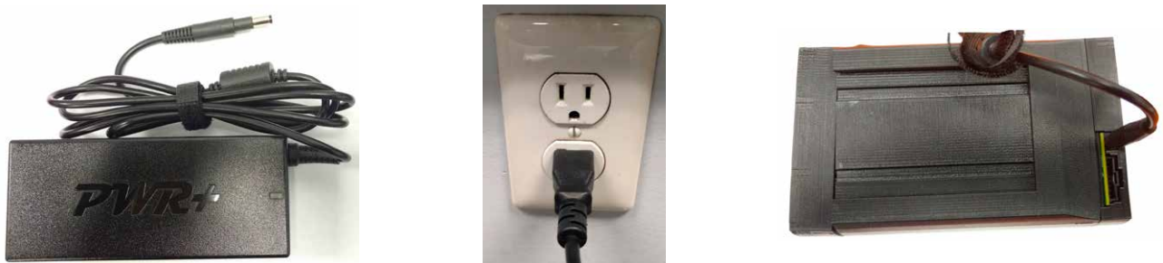
Figure 1.7 - DC power adapter (left) plugging into a wall outlet (middle), and then into the smart battery pack (right)
